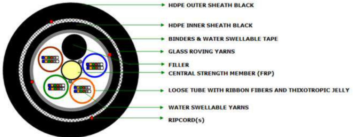
TYPICAL STRUCTURAL DRAWING FOR 96 FIBRE OF DRY CORE CABLE
