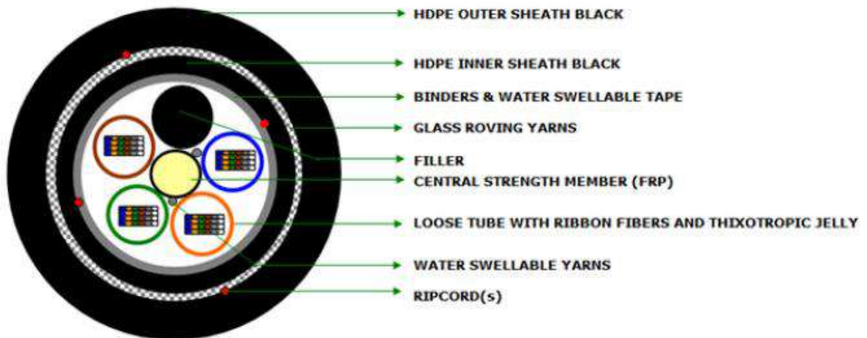
TYPICAL STRUCTURAL DRAWING FOR 96 FIBRE OF DRY CORE CABLE
