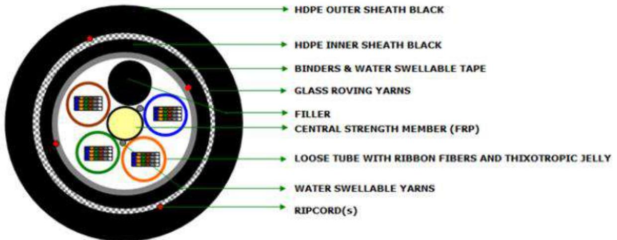
**3.9.1 Secondary Protection:** The primary coated Ribbon fibres may be protected by loose packaging within tube, which shall be filled with thixotropic jelly. The dimensions of tube shall be as per Table – I above.
