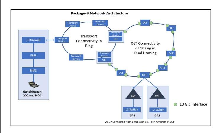
3.2 In a present network, physical connectivity between 2 layers of transport mux and transport switch/OLT is as per below in both packages.
