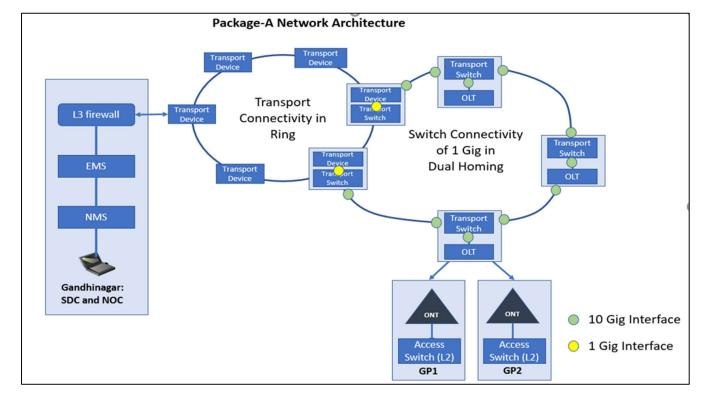
**Note:** Average 20 GP (Gram Panchayat) connected from 1 OLT (Optical Line Terminal) with 2 GP per PON (Passive Optical Network) Port of OLT. In few OLTs, approximately 25-27 GPs connected.
